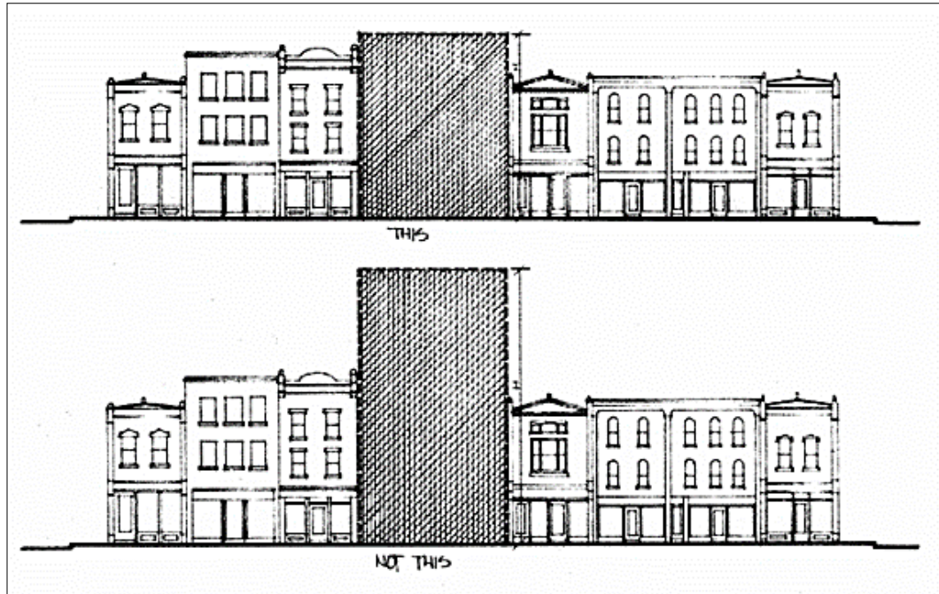
Figure 15.07.50b: Building Height Example
