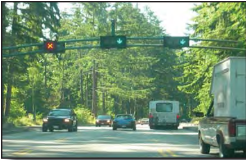
Figure 5-10 Reversible lane signalization
