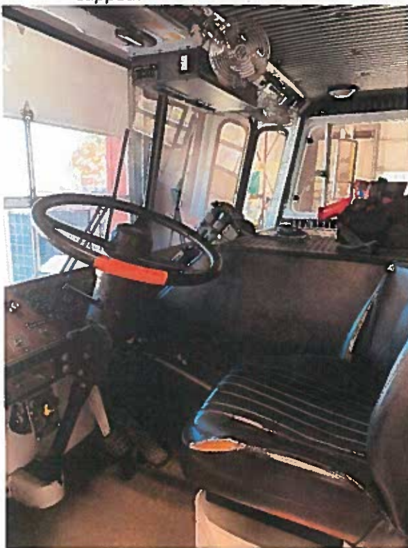
Cab: Damaged steering wheel and Vinyl seats.
