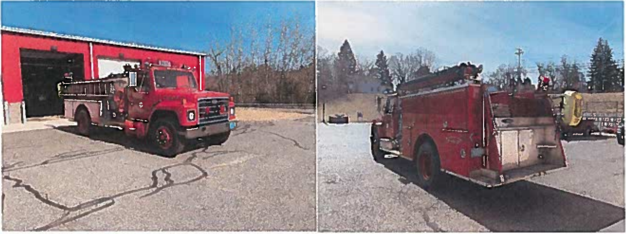
Engine 2, 1987 500 GPM pumper International Chassis
