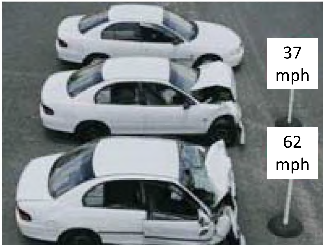
Figure 4.5: Difference in deformation striking a solid object at 60 km/h and 100 km/h
