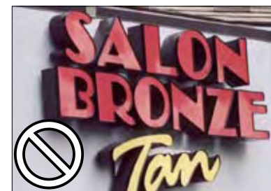
Internally-lit plastic-front channel letters.
