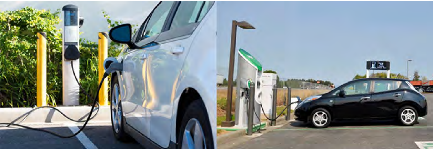
Level 2 chargers (left) are common in home, workplace, and public settings and can charge a BEV from empty in 4-10 hours. Direct current fast chargers (right) are common as public chargers and along highway corridors and can charge a BEV to 80 percent in under an hour. (123RF and Washington State Department of Transportation photos)
