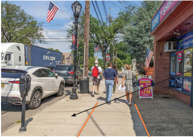
2+ Feet Utility Zone 5+ Feet Pedestrian Zone 2+ Feet Frontage Zone
