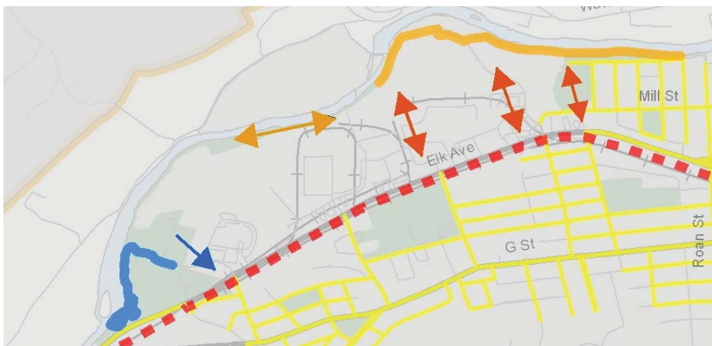
Primary objectives for non-motorized travel should include: (1) taking advantage of large parcels and undeveloped or redeveloping lands along the river to extend the Linear Path (orange), (2) finding a connection between the Rails to Trails corridor and Sycamore Shoals (blue), and (3) planning for connections between the Rails to Trails corridor and the extended Linear Path (red).
