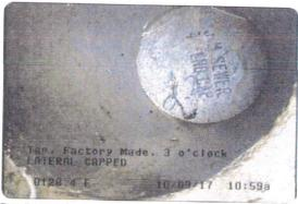
Tap, Factory Made at 128.4 feet, 3 o'clock, 4 in | LATERAL CAPPED
