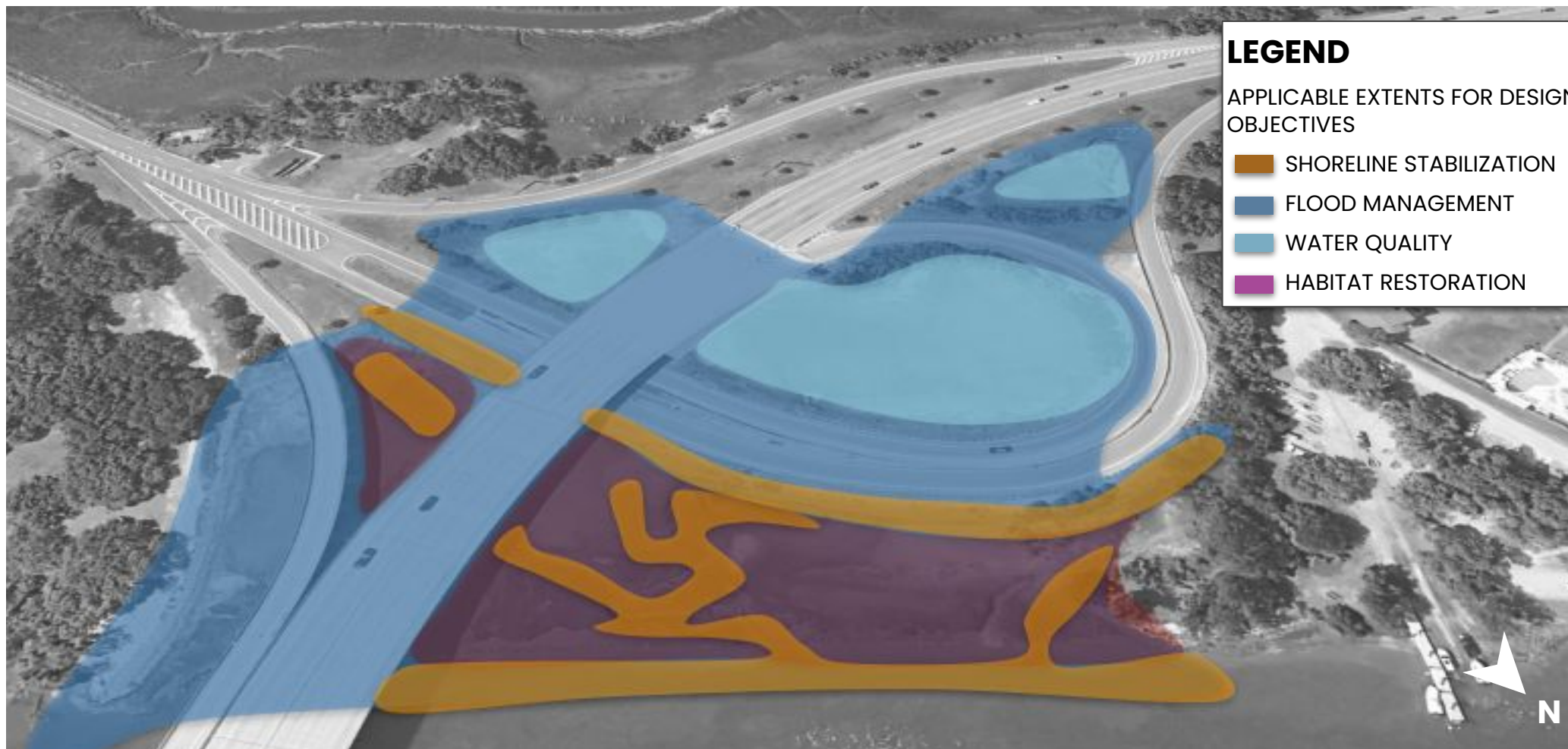
Figure 1.6. Spatial Extents of MIRR-Identified design objectives for the Shell Point Interchange across the site.
