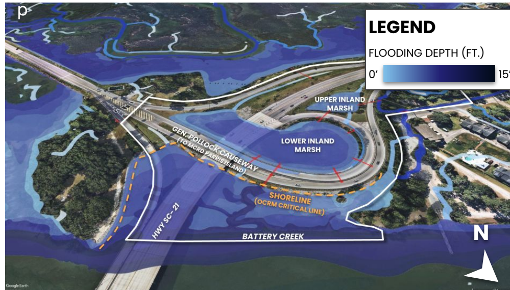
Figure 3.3. Anticipated inundation extents result from a 2045 high-tide flood coinciding with rainfall patterns experienced during Hurricane Debby (2024). Surface drainage patterns also shown to indicate how water accumulates in the absence of pipes.
