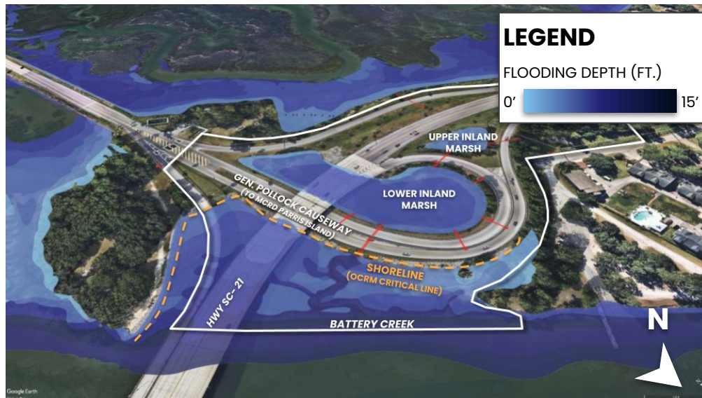
Figure 3.2. Inundation depths anticipated across the site resulting from a high-tide flood that occurs 30x per year in 2035.
