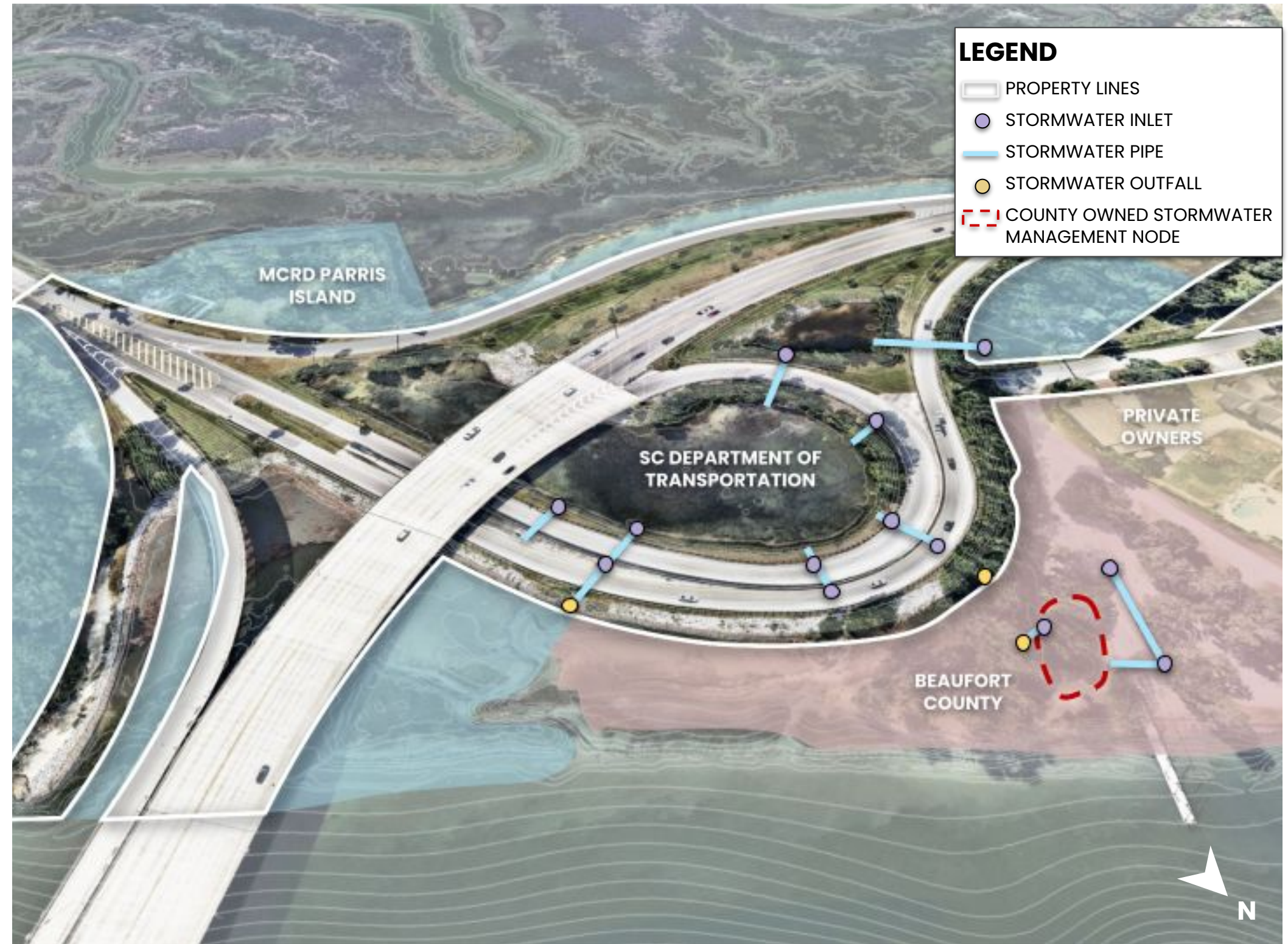
Figure 1.5. Context map of the Shell Point Interchange highlighting property lines, delineation of jurisdictional wetland extents, and existing utility infrastructure.
