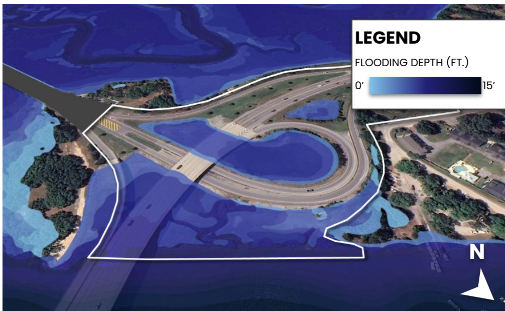
Figure 2.11. Inundation extents of 10-yr AEF in 2025 (i.e., storm with 10% statistical probability of occurring at site in any given year)
