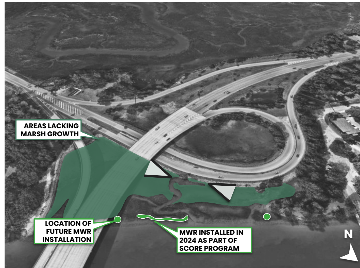
Figure 4.3. Extents of areas lacking marsh growth with corresponding site photos; Planned extents of Manufactured Wire Reefs to be installed
