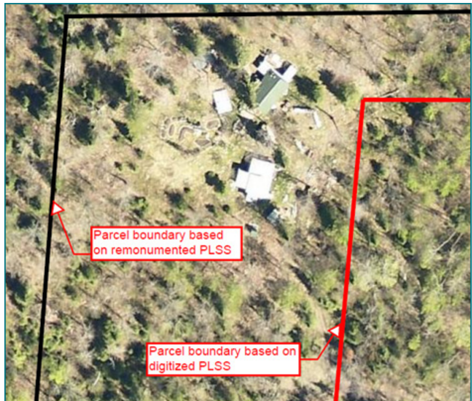
The image above shows an area where parcel representation was spatially inaccurate due to the lack of PLSS remonumentation. When the PLSS was remonumented in the area, the parcel map was updated to more accurately reflect conditions on the ground.
