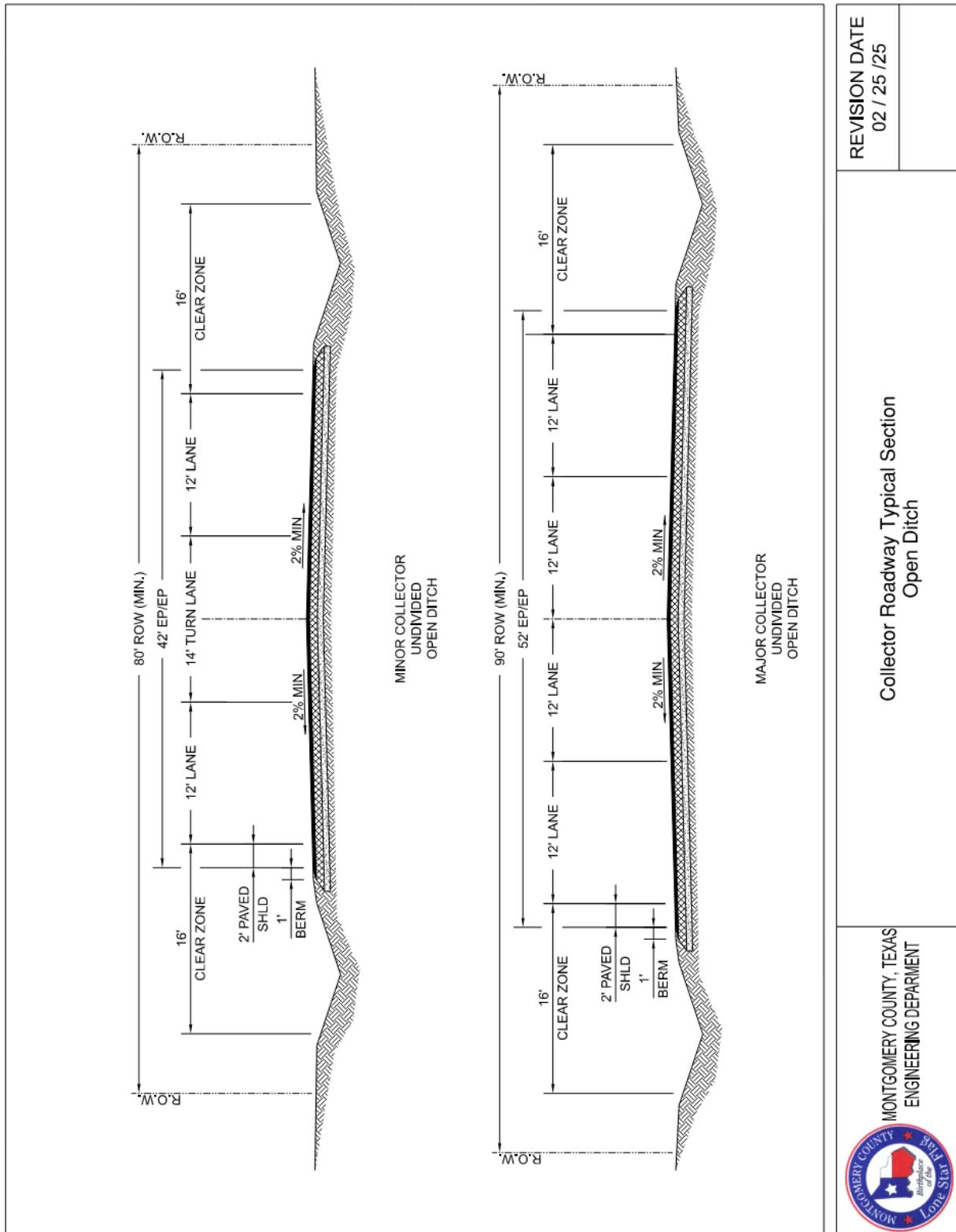
**F. COLLECTOR/THOROUGHFARE ROADWAY TYPICAL SECTION (OPEN DITCH)**
