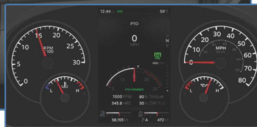
Standard Instrument Panel with 7-Inch Digital Display
