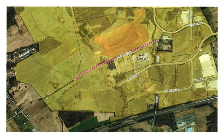
Howard Allen Road varies in width from west to east approximately ten feet, from a right-of-way width of 30 feet to 50 feet then to a 40 foot right of way nearing Witt Road. Approximately 3,500 linear feet of this street from the corporate limits to its terminus with Witt Road is needed to be vacated in order to construct the Parkway extender.
