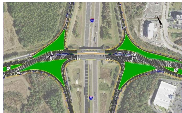
Florida DOT Diverging Diamond Interchange currently under construction at SR 56 and I-75.
