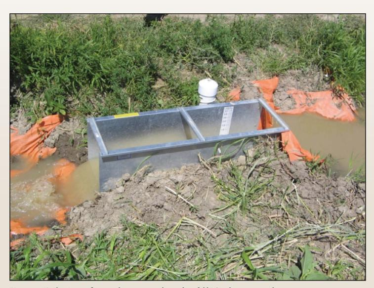
**Figure 12.** EZ Flow Ramp™ flume used to measure tailwater from field DS14 during 2005 and 2007
