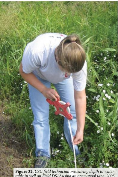
table in well on Field DS12 using an open-spool tape, 2005
