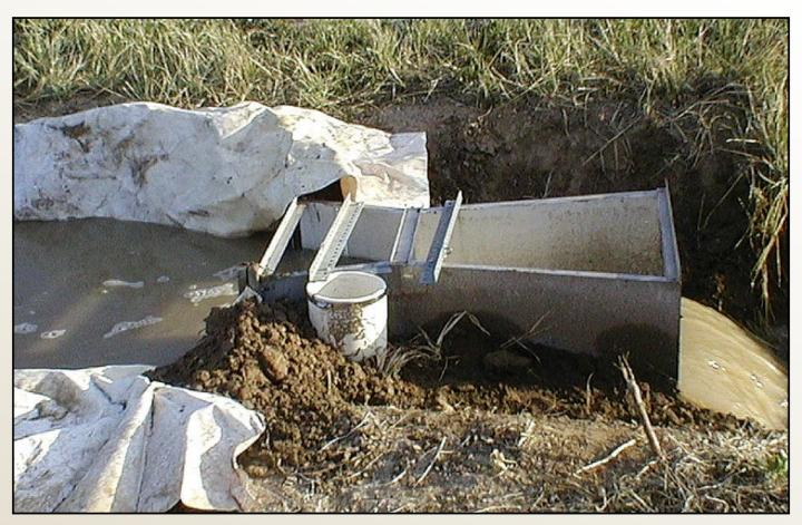
Figure 15. Cutthroat flume for measurement of tailwater runoff from field US14C in 2008
