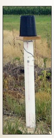
**Figure 20.** HOBO\* rain gauge in Field US17E in 2008
