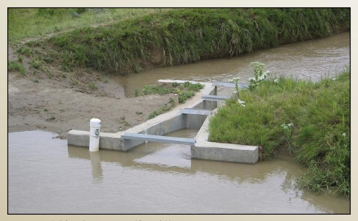
**Figure 16.** Parshall flume for measurement of flow to field DS1 in 2008
