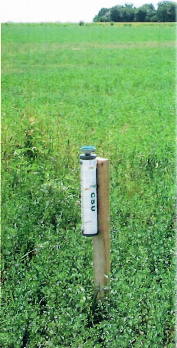
Figure 22. ETgage® Model A atmometer in field DS2 during the 2006 season
