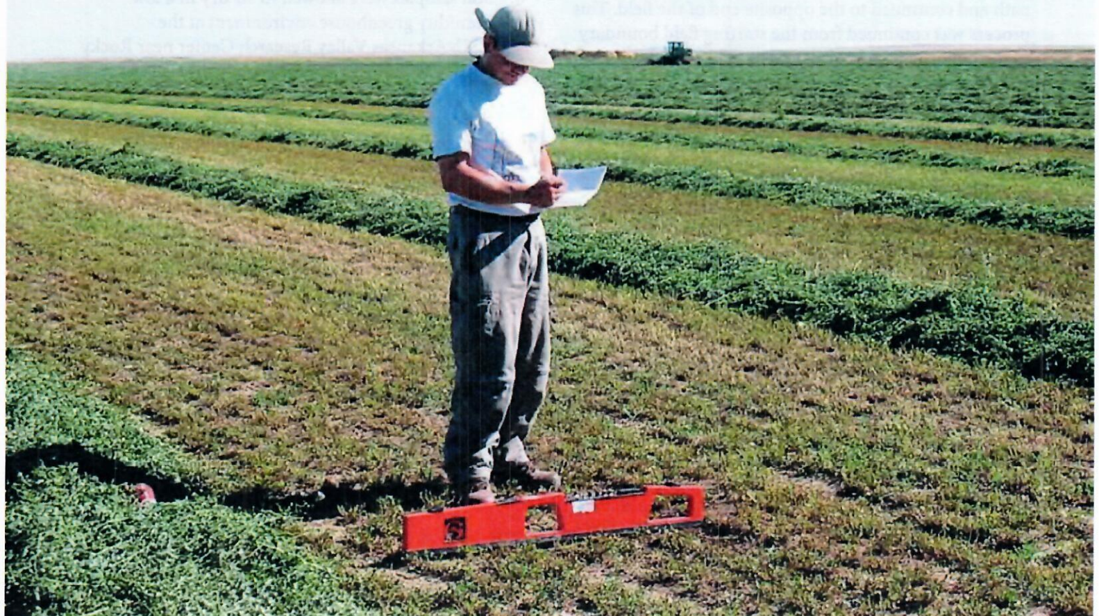
Figure 33. CSU technician conducting EM38 survey on a field in the LARV
