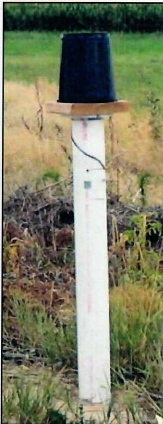
Figure 20. HOBO® rain gauge in Field US17E in 2008
