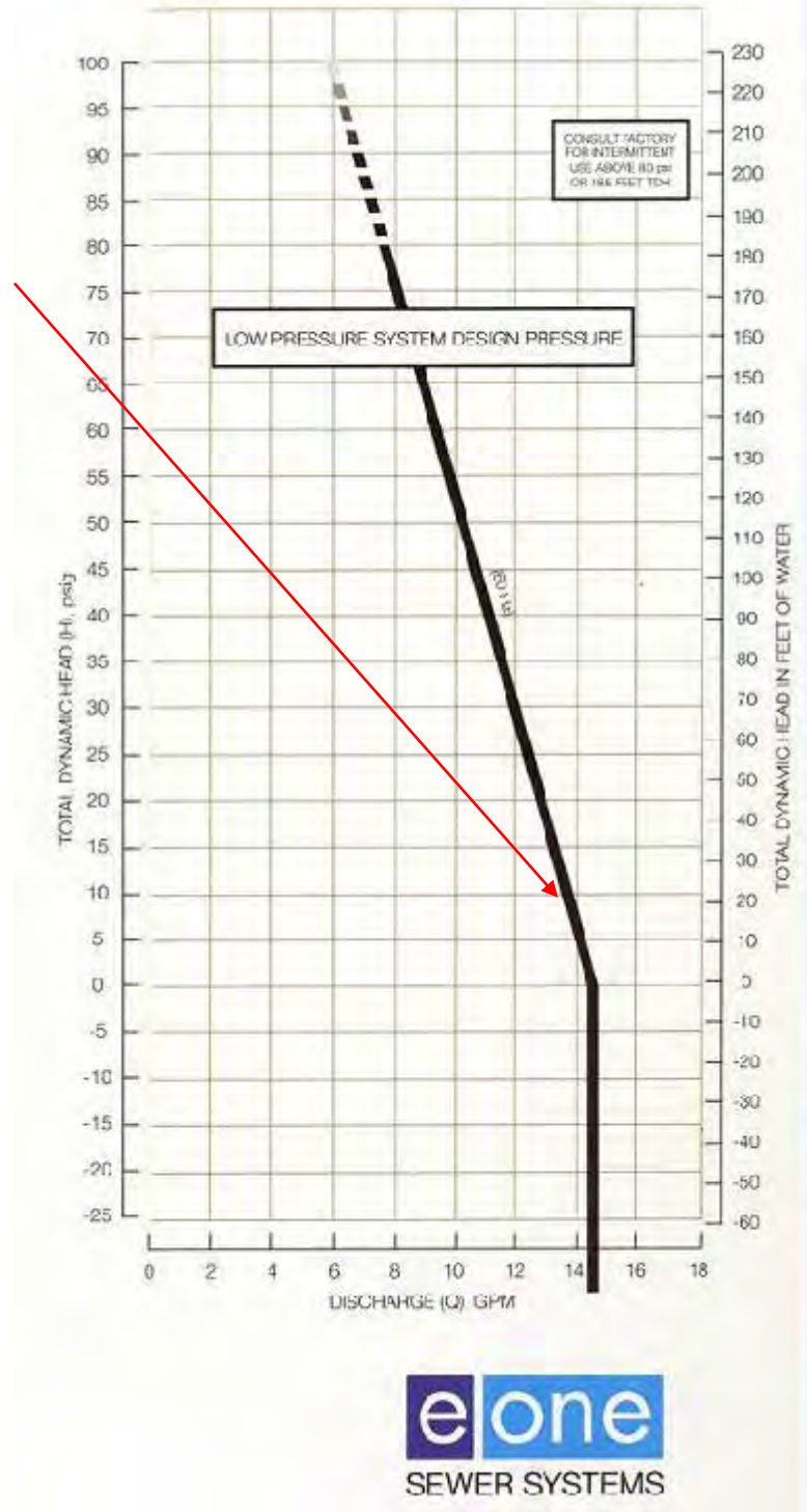
GRINDER PUMP PERFORMANCE CHARACTERISTICS
