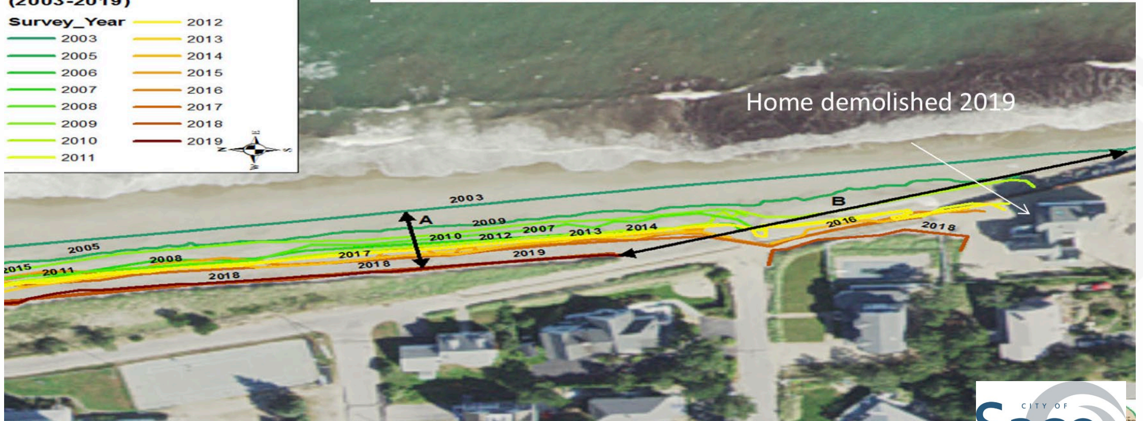
Figure 1. Dune shorelines along Ferry Beach, Saco from 2003 to 2019 show that the seaward dune edge eroded approximately 67 feet (Arrow A), a rate of -4.2 feet/year. The southern tip of the dune migrated northwards about 321 feet (Arrow B), a rate of about 20 feet/year. 2003 shoreline position from aerial photo interpretation. 2005-2019 shoreline positions from the MGS Maine Beach Mapping Program. 2018 NAIP Base Imagery.
