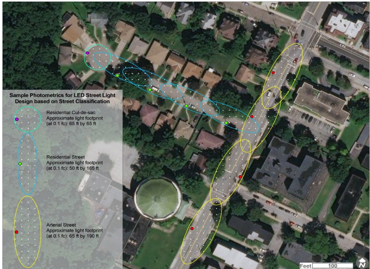
Examples of the different distribution pattern requirements based on roadway classification.
