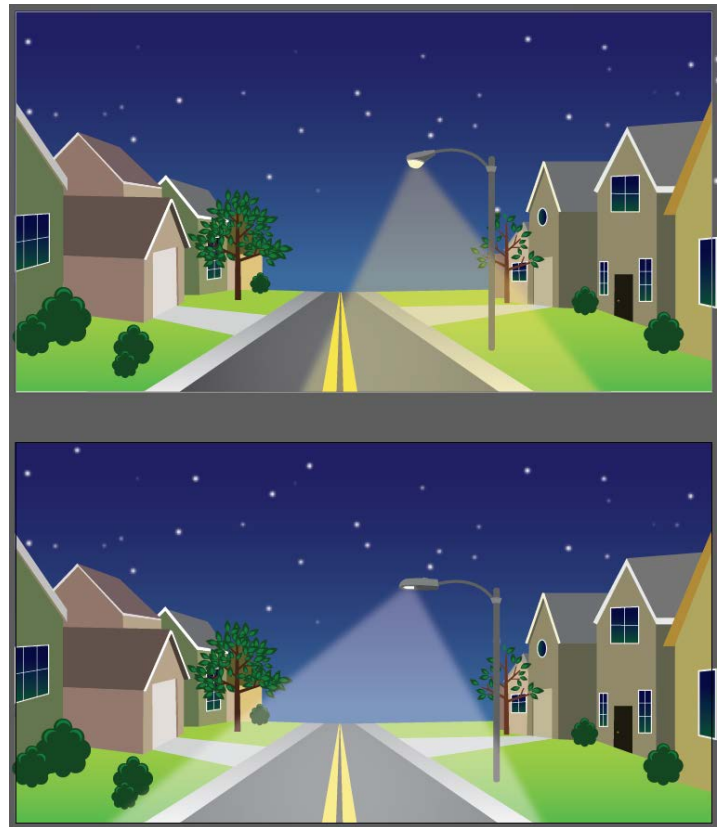
Figure 2: Examples of the different light distribution patterns from an HPS fixture (top) vs. an LED fixture (bottom).
