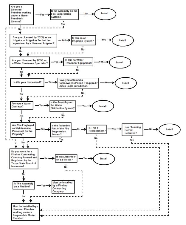
*Note:* All backflow prevention assemblies must be tested by a licensed BPAT upon installation.
