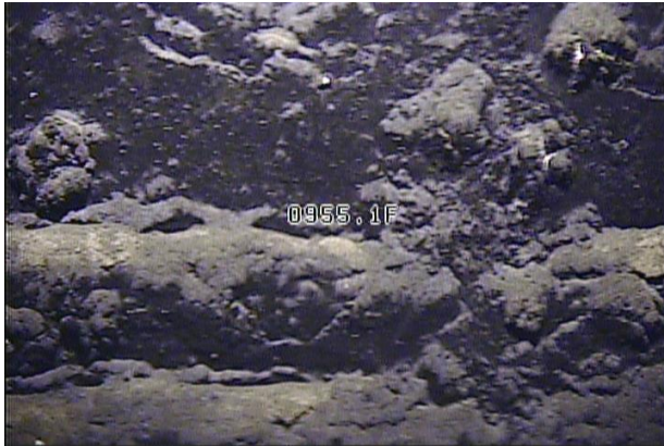
Casing slots at 955 ft bgl top of screened interval with heavy precipitation
