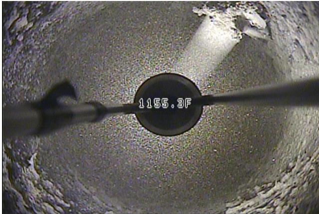
Broken sample pipe piece top at 1157 ft bgl
