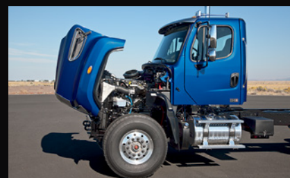
Full tilt hood for easy engine access.
