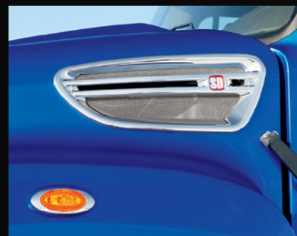
Engine air intake with pre-cleaner for dusty environments.
