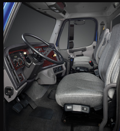
Ergonomically designed driver's area features an automotive-style dash, easy-to-read LED-backlit gauges and controls within easy reach.
