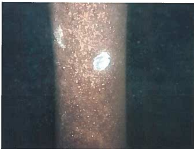
59 Support Column Having Good Adhesion Value Of The Coating And A Heavy Stain To A Film Of Precipitate
