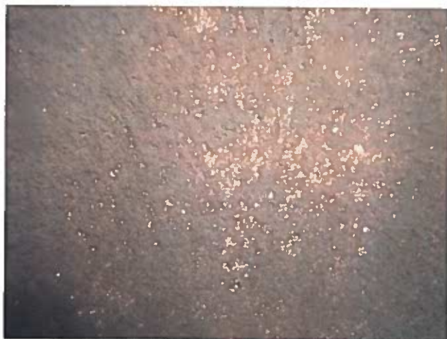
45 Interior Wall Having A Heavy Stain To A Film Of Precipitate
