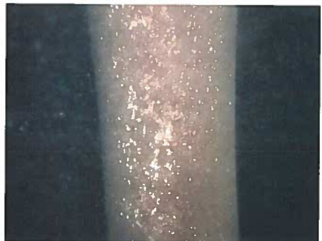
60 Support Column Having Good Adhesion Value Of The Coating And A Heavy Stain To A Film Of Precipitate
