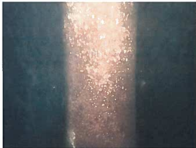
63 Support Column Having Good Adhesion Value Of The Coating And A Heavy Stain To A Film Of Precipitate
