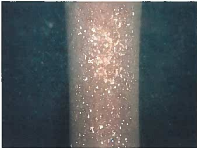
61 Support Column Having Good Adhesion Value Of The Coating And A Heavy Stain To A Film Of Precipitate
