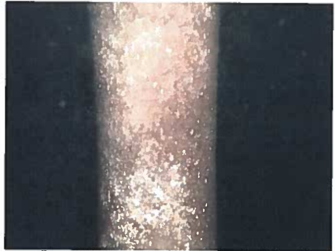
58 Support Column Having Good Adhesion Value Of The Coating And A Heavy Stain To A Film Of Precipitate
