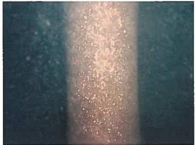
62 Support Column Having Good Adhesion Value Of The Coating And A Heavy Stain To A Film Of Precipitate
