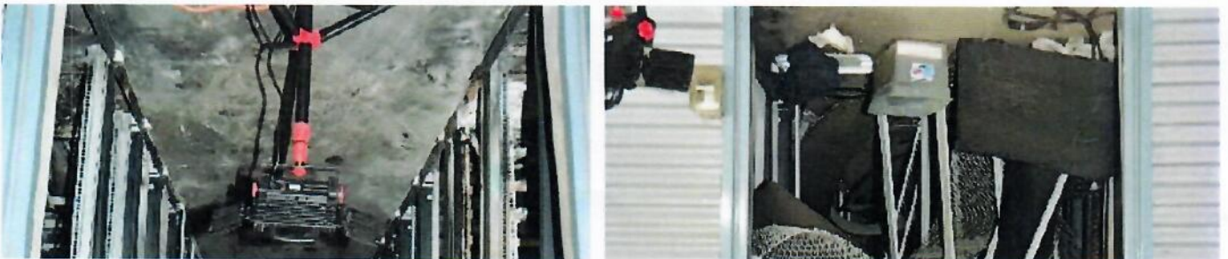
Interior damage to the BESS after the explosion [left], and after debris was removed to gain access to begin the forensics analysis [right]. PHOTOS: ARIZONA PUBLIC SERVICE
