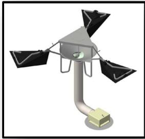
The first SolarBee Recirculation System introduced to the market is an active type system that consists of a solar powered pump that floats on the water surface in the center of the storage tank. The intake for the pump is set just above the tank floor and is curved upward to reduce the potential for redistributing the sediment that has settled on the bottom of the tank. Water is drawn from the lower portion of the tank and distributed at the water surface to promote mixing in the tank.
