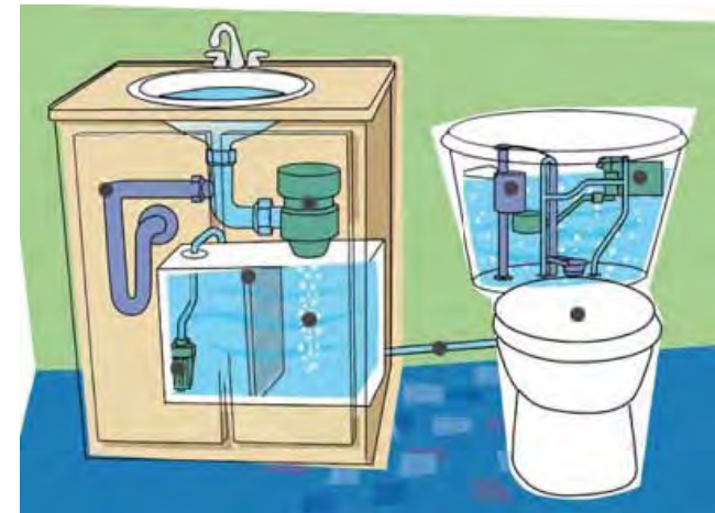
Figure 98: Example of potential wastewater reuse. The AQUUS® system takes wastewater from a bathroom sink and diverts it through a filtration system to the toilet to be used for flushing the toilet.
