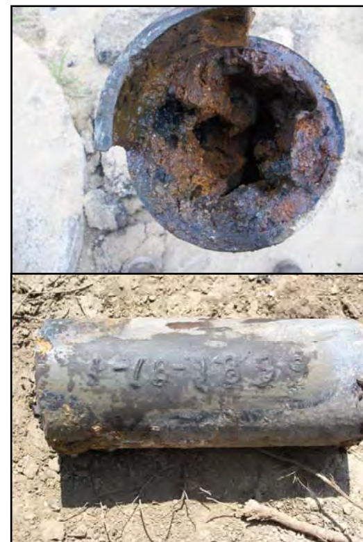
Figure 95: Tuberculated water pipes. Tuberculated pipes reduce household water pressure, and affect fire hydrant flows and water quality. Some of Ware's infrastructure is over 100 years old. Bottom photo shows a water pipe from 1899 which was replaced in 2013.
