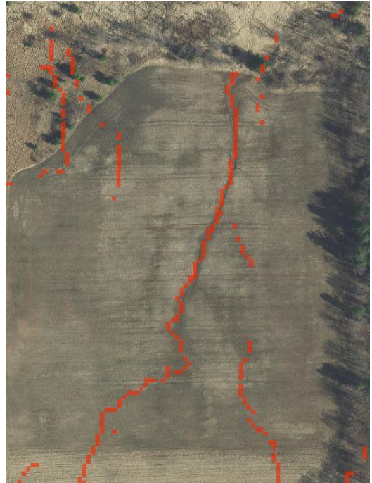
Figure 31. High stream power index indicating potential gully erosion.
